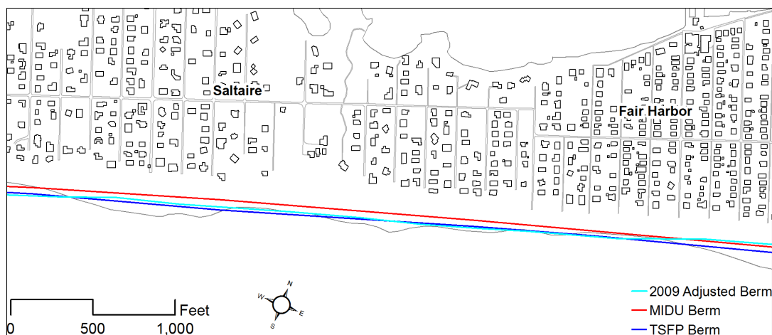
Figure 8-7. 2009 Design Berm at Western Fire Island
