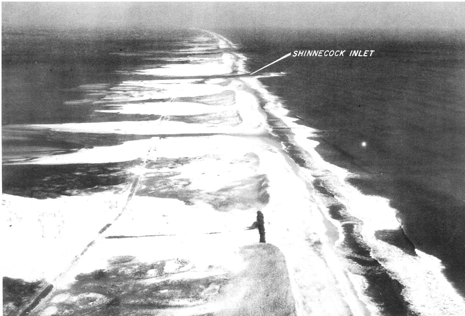
Figure 2-1. Extensive overtopping of dunes and breaks through the barrier island east of Ponquogue Bridge during the hurricane of September 21, 1938. Shinnecock Inlet, which opened during the storm is shown in the photo.
