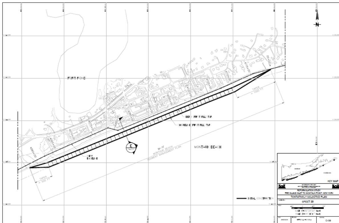
Figure 30. Montauk Beach Feeder Beach location and typical Sediment Management Construction Template
