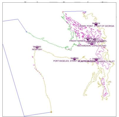
Figure C1 – Example of a TCARI grid boundary Tidal datum locations as well as active water level gauge sites are applied, and a triangular network is created to enable the constituent and residual interpolation (Fig C2).
