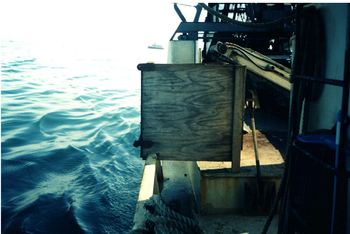
Photograph 8 – Calibrated Hopper Used for Catches Exceeding 25 Bushels
