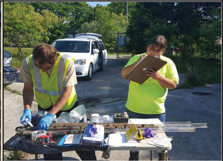
Photo 4. AECOM and CGE completing lithologic logging and sample collection from soil boring at FPH.
