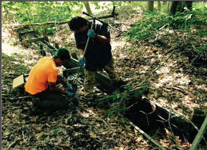
Photo 3. AECOM and New England Geotech collect samples via hand-auger at H-22.
