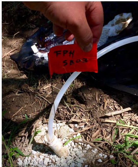
Fuel Pump House/AST 35. Location FPH-SB03 had elevated PID readings in soil and the temporary well headspace and petroleum odor in purged groundwater, June 2016.
