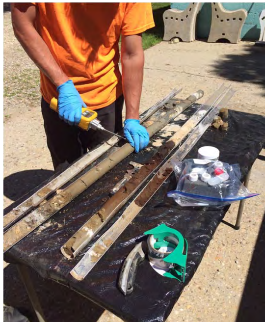
Motor Pool. John Hudson (CGE) completing PID screening of the soil core from MP-SB01, the location within the Motor Pool garage bay, June 2016.
