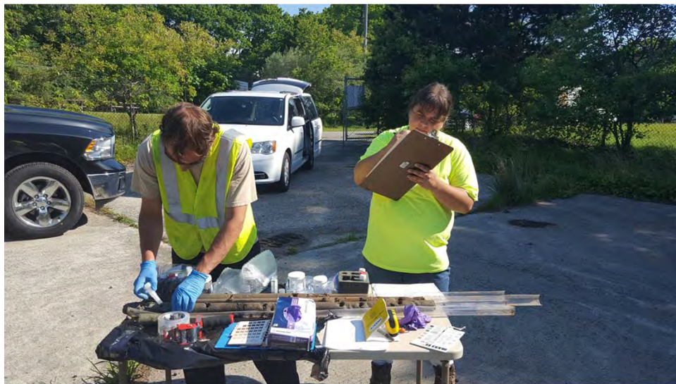
Fuel Pump House/AST 35. Nicole Schulman (AECOM) completing soil logging at AST35-SB03 while John Hudson (CGE) collects soil samples, June 2016.
