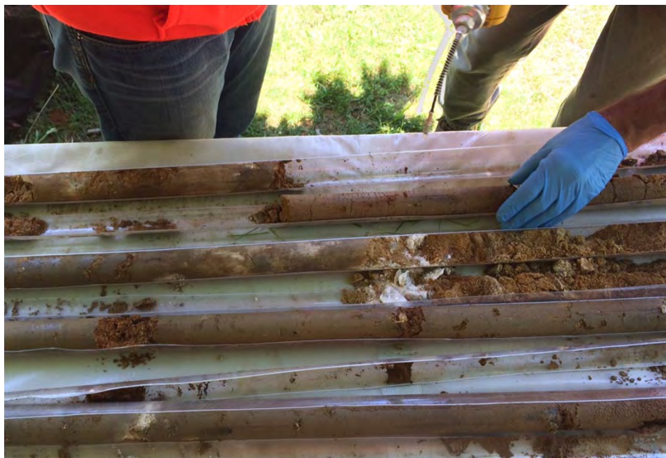
Waste Disposal System. Soil cores at location WDS-SB14, including the first four runs (0 to 20 ft bgs), June 2016.
