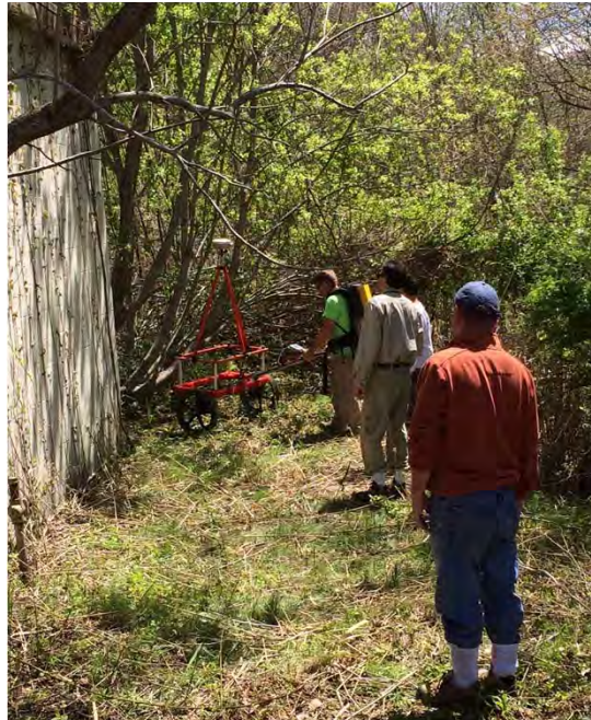
Fuel Pump House/AST 35. Geophysical survey around the Fuel Pump House to identify former fuel distribution line, May 2016.
