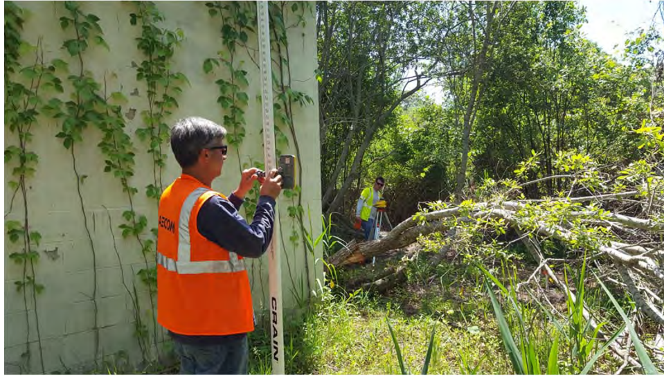
Fuel Pump House/AST 35. Collection of temporary well location surface elevations by the Clean Globe Environmental (CGE) land surveying team, June 2016.
