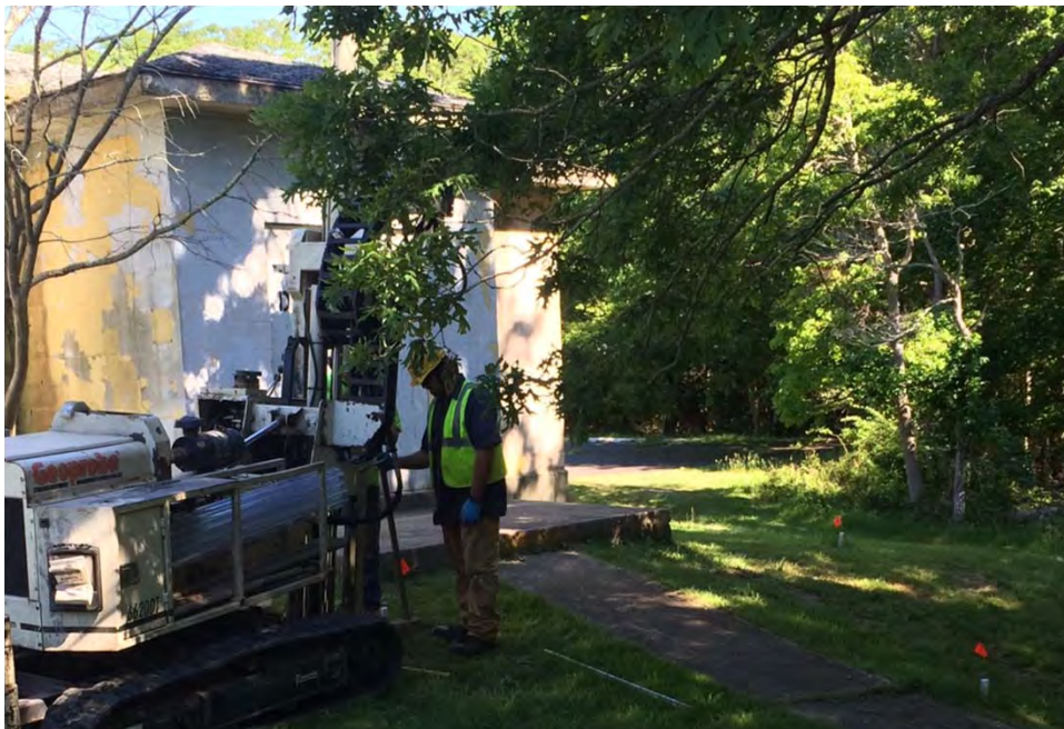
Suspected Tank B (Building 22). Mike Podamy (NEG) conducting soil borings around Suspected Tank B via Direct Push rig 6620DT, June 2016.
