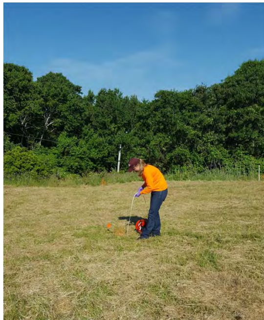
Former Building 203. Location PZ-03 at former Building 203 being gauged with an interface probe; five feet of free product was identified on 17 June 2016.
