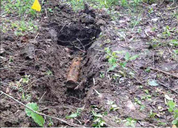
Photo 1. The Fuel Pump House distribution was located with the magnetometer. Hand-digging indicated that the line had been cut and removed after approximately 6-feet from the fuel house.
