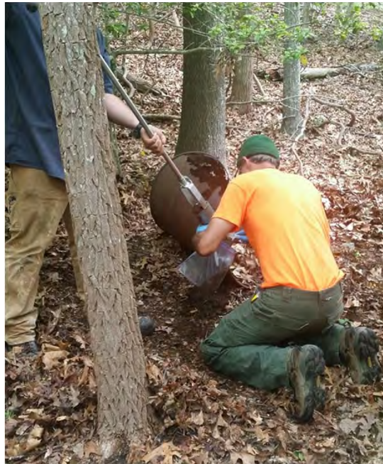
H-3. Surface soil sample collection at H-3 via hand auger, June 2016.
