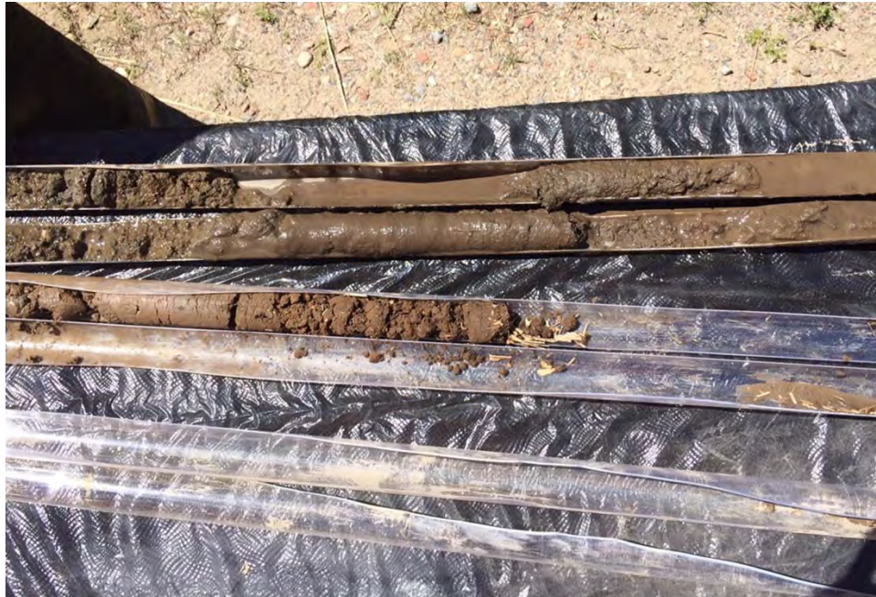
Waste Disposal System. Re-collection of the WDS-SB01 0 to 5 ft bgs run, which yielded more recovery than the initial run; still wet/mucky near surface, June 2016.
