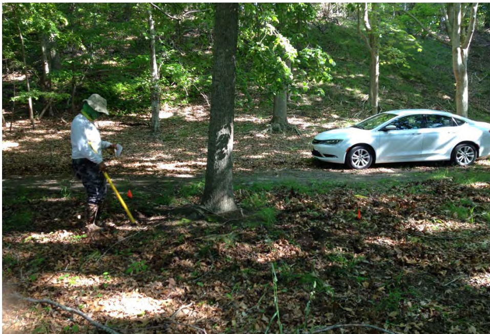
H-18. UXO Technician II LeNina Bennerson (AECOM) performs a magnetometer survey of H-18; there was no drum at this location but metal debris were identified, June 2016.
