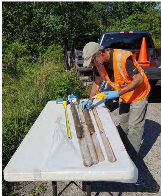
Fuel Pump House/AST 35. Geologist Mike Glinski (AECOM) performing PID-screening of soil cores from location FPH-SB01, June 2016.
