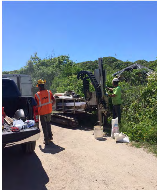
Waste Disposal System. Soil core collection from location WDS-SB03 by the chlorine contact chamber via the Direct Push 6620DT rig by Keith Precious (NEG), June 2016.
