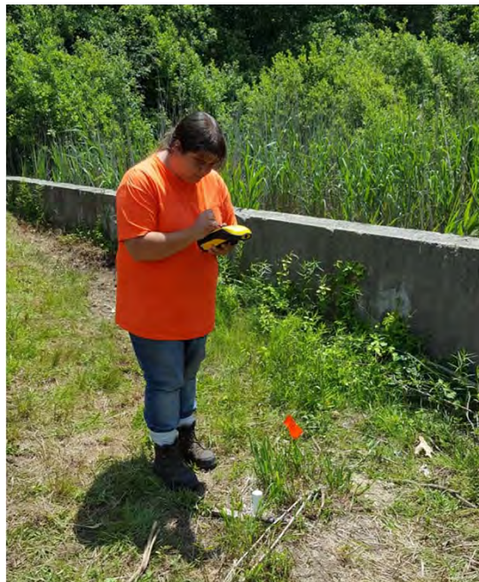
Fuel Pump House/AST 35. Sample location coordinate collection using the Global Positioning System Trimble GeoXH unit, June 2016.
