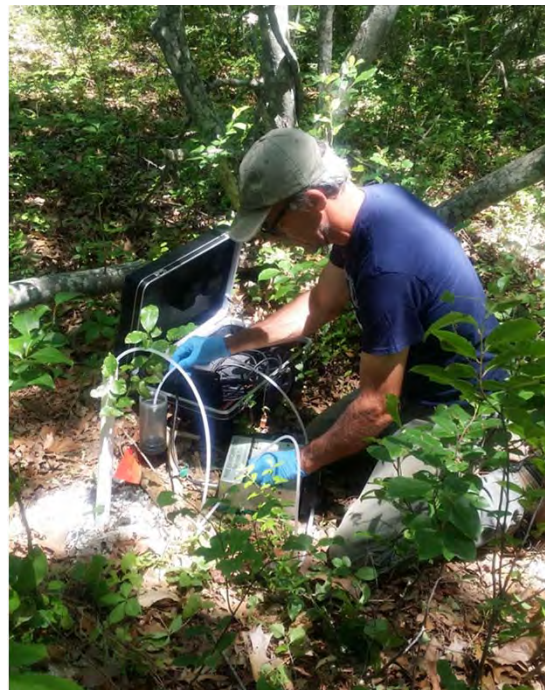
Mike Glinski (AECOM) collecting groundwater samples.
