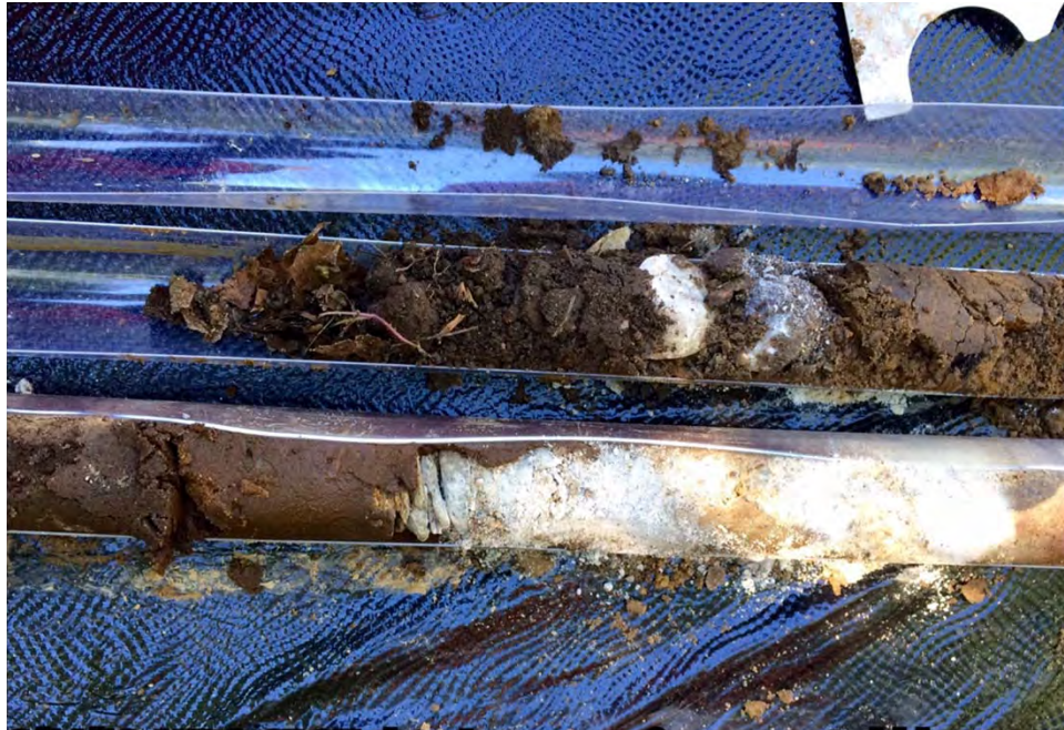
Waste Disposal System. Soil core from location WDS-SB07 showing zone of concrete rubble around 6.5 to 7 ft bgs, June 2016.
