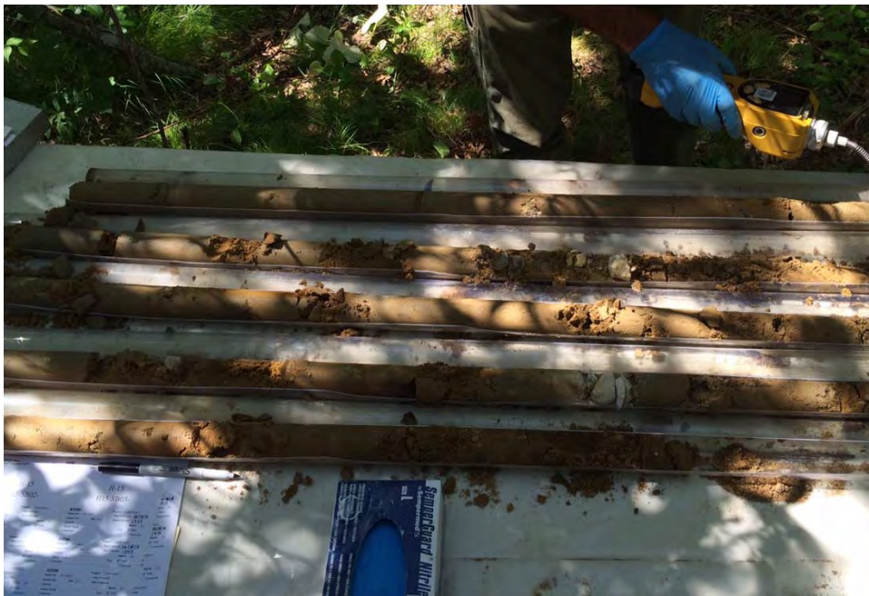
H-15. Soil cores from location H15-SB02, from 0 to 25 ft bgs, with very slight moisture noted from 15 to 25 ft bgs, June 2016.
