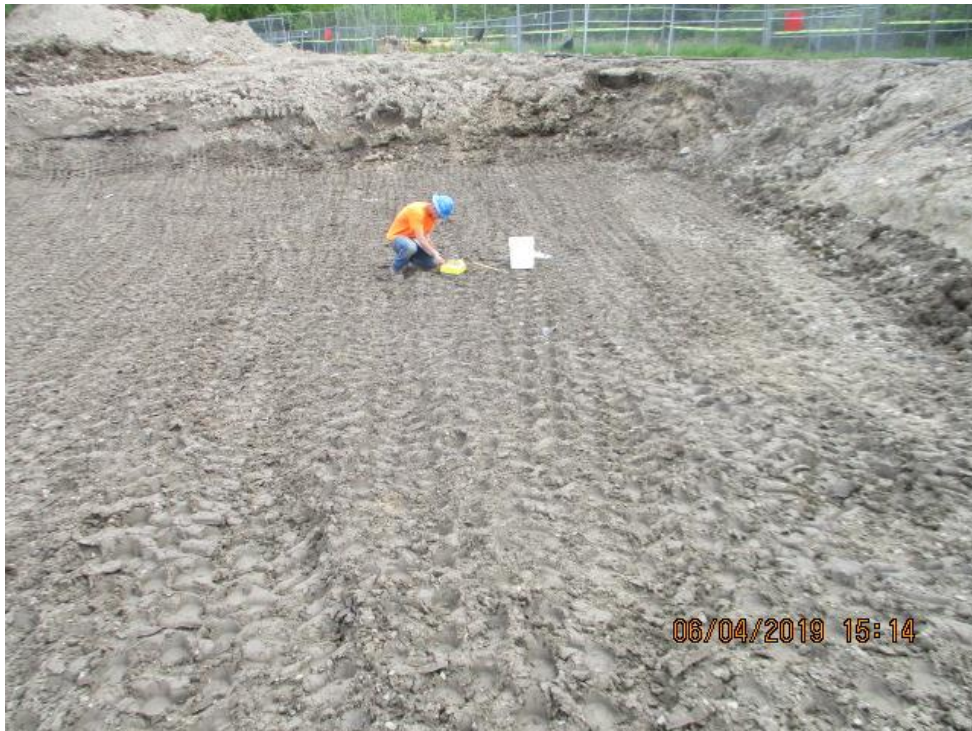
Photograph 45: Backfill compaction testing at Silo 5 (06/04/19).
