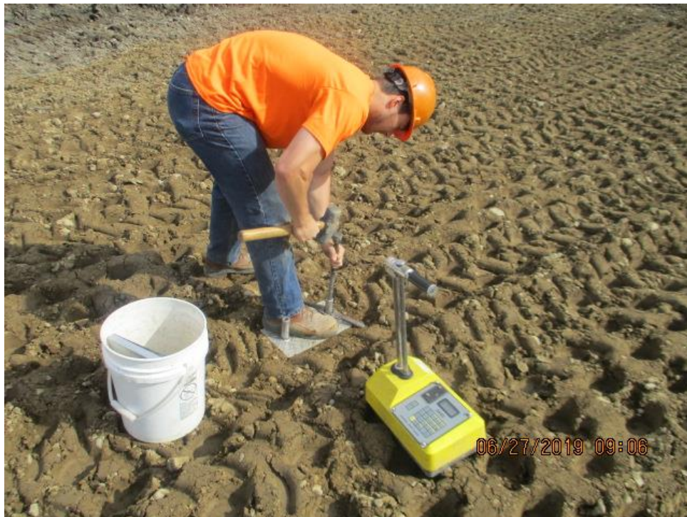
Photograph 48: Backfill compaction testing (06/27/19).
