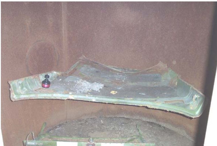
Tank Interior 1 – A radon electret is visible on the left. The Saab hood is sitting on the rack at the rear of the tank
