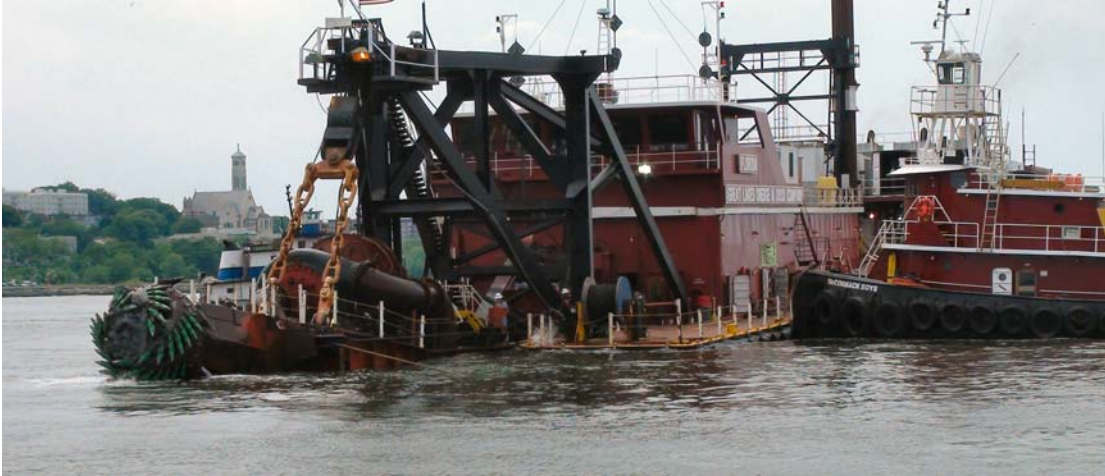
Figure 1. The dredge Florida with attached HP Esco 54D cutterhead.
