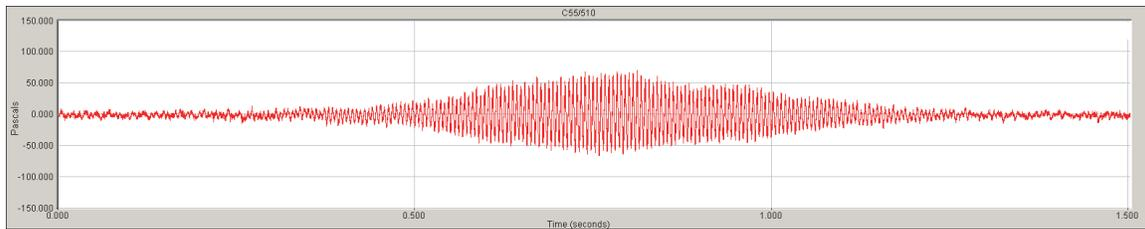
Figure 16. Pressure waveform for spud “walking” sounds.
