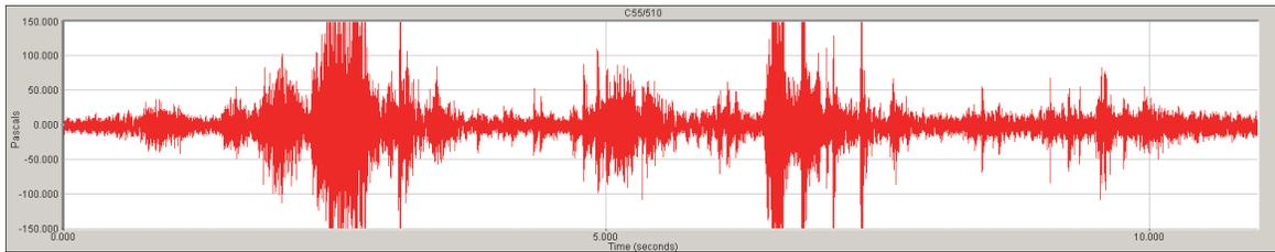
Figure 6. Pressure waveform for bottom grab (scoops) sounds.
