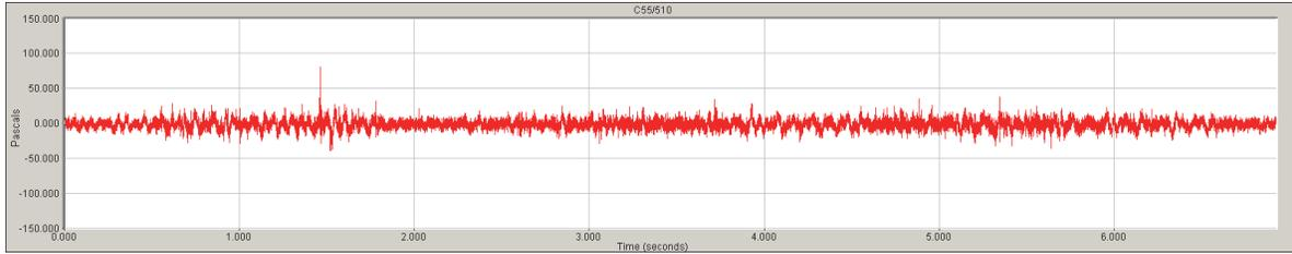
Figure 12. Pressure waveform for barge loading noise.
