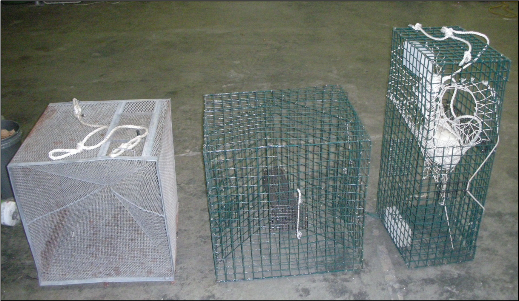
Figure 2. Sampling gear deployed during the Ambrose Obstruction Biological Sampling including the single fyke fish trap with \frac{1}{4} -inch wire mesh (left), the double fyke 24-inch x 24-inch x 24-inch crab pot (center), and the double fyke 36-inch x 18-inch x 12-inch lobster pot (right), September 2009.
