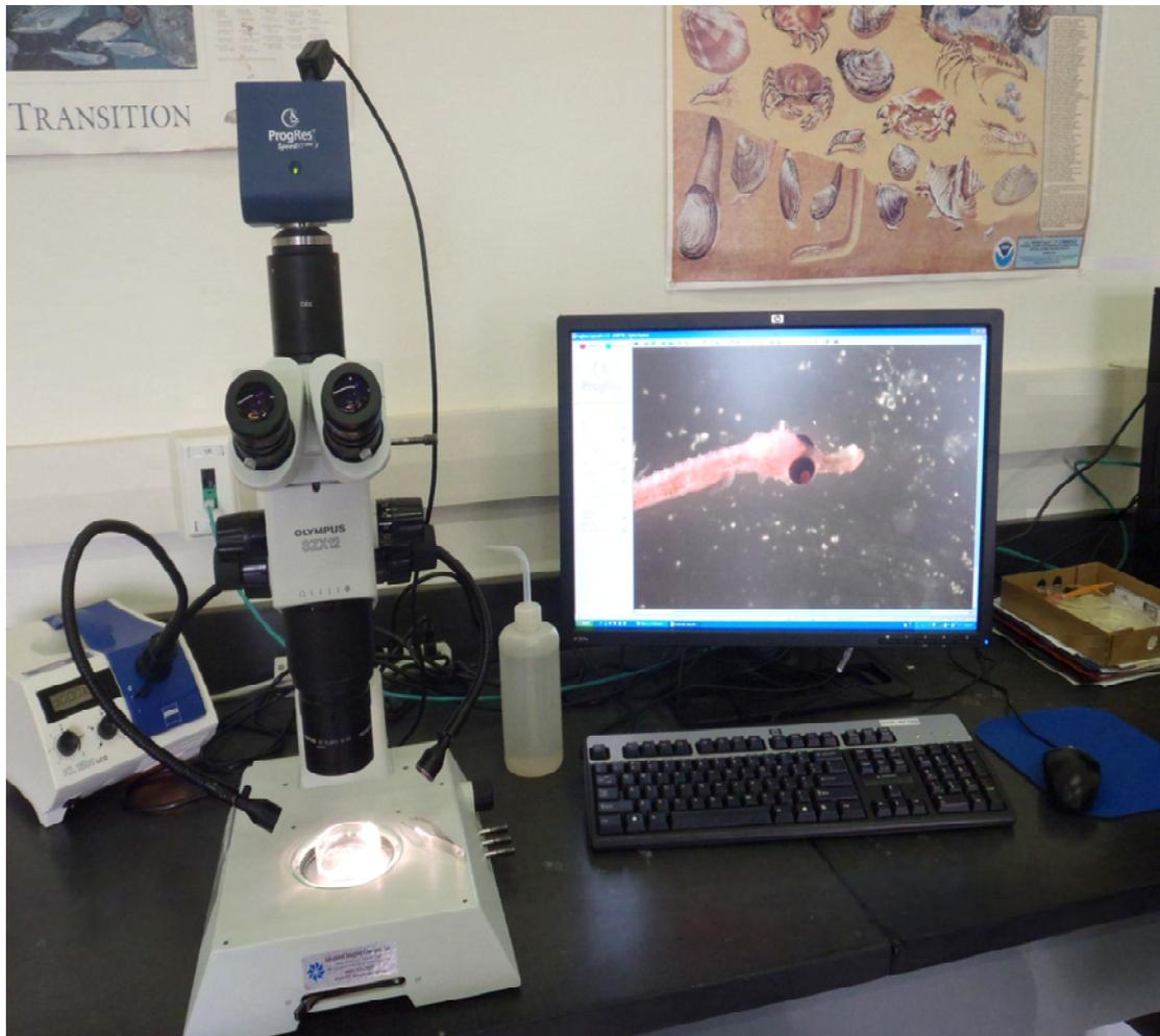
**Figure D-1. Laboratory analysis set up showing the Jenoptik ProgRes CapturePro 2.8.0 Camera and Olympus SZX12 Tri-Ocular Stereo Microscope.**
