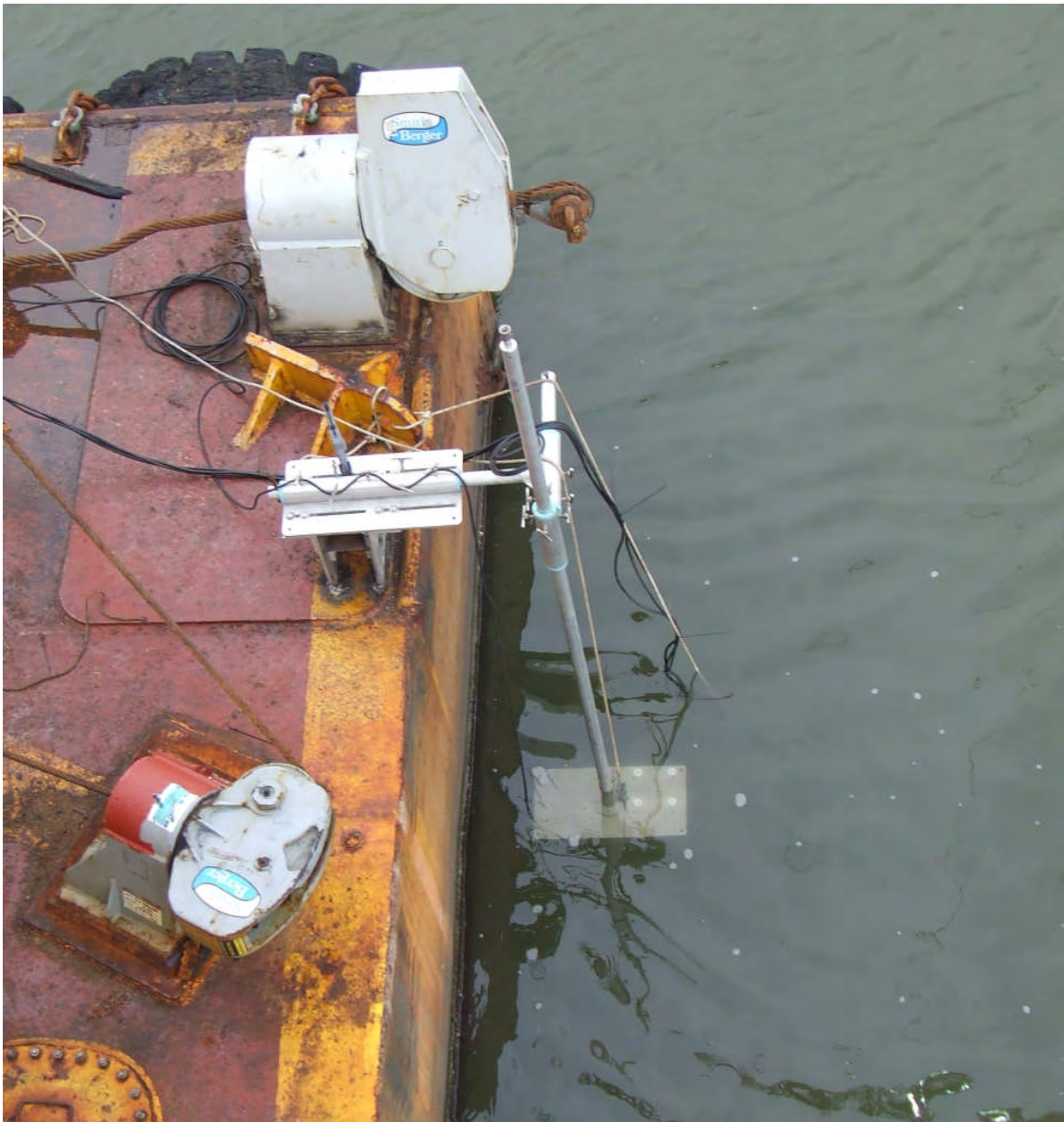
Figure 8. Location of sensors deployed from the dredge platform. The vertical tube supports the ADCP transducer assembly just below the water's surface. A string of three OBS units was deployed outboard from the ADCP mount.
