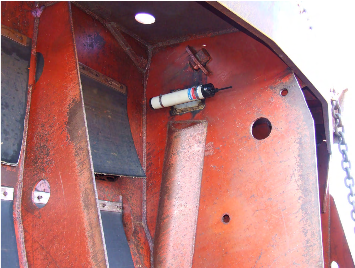
Figure 31. Location of OBS instrument on the outboard side of the bucket.
