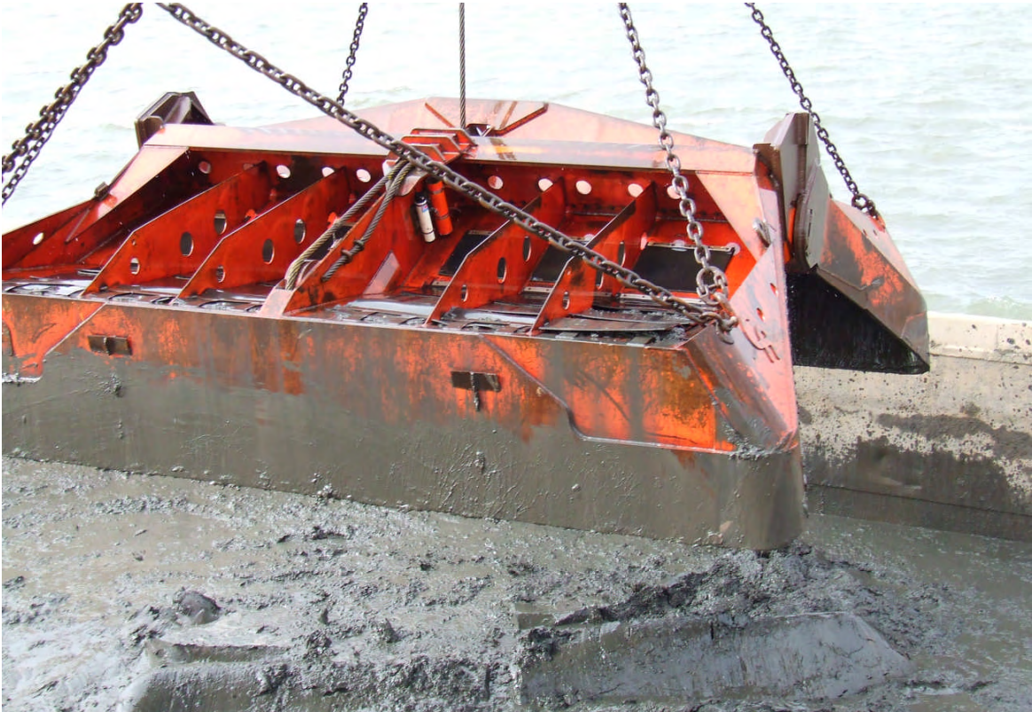
Figure 7. Sensor location. The orange accelerometer canister and white OBS housing are visible attached to the bucket's central support rib. This sensor array is on the "inboard" side of the bucket, which always faces the derrick and operator's cab.
