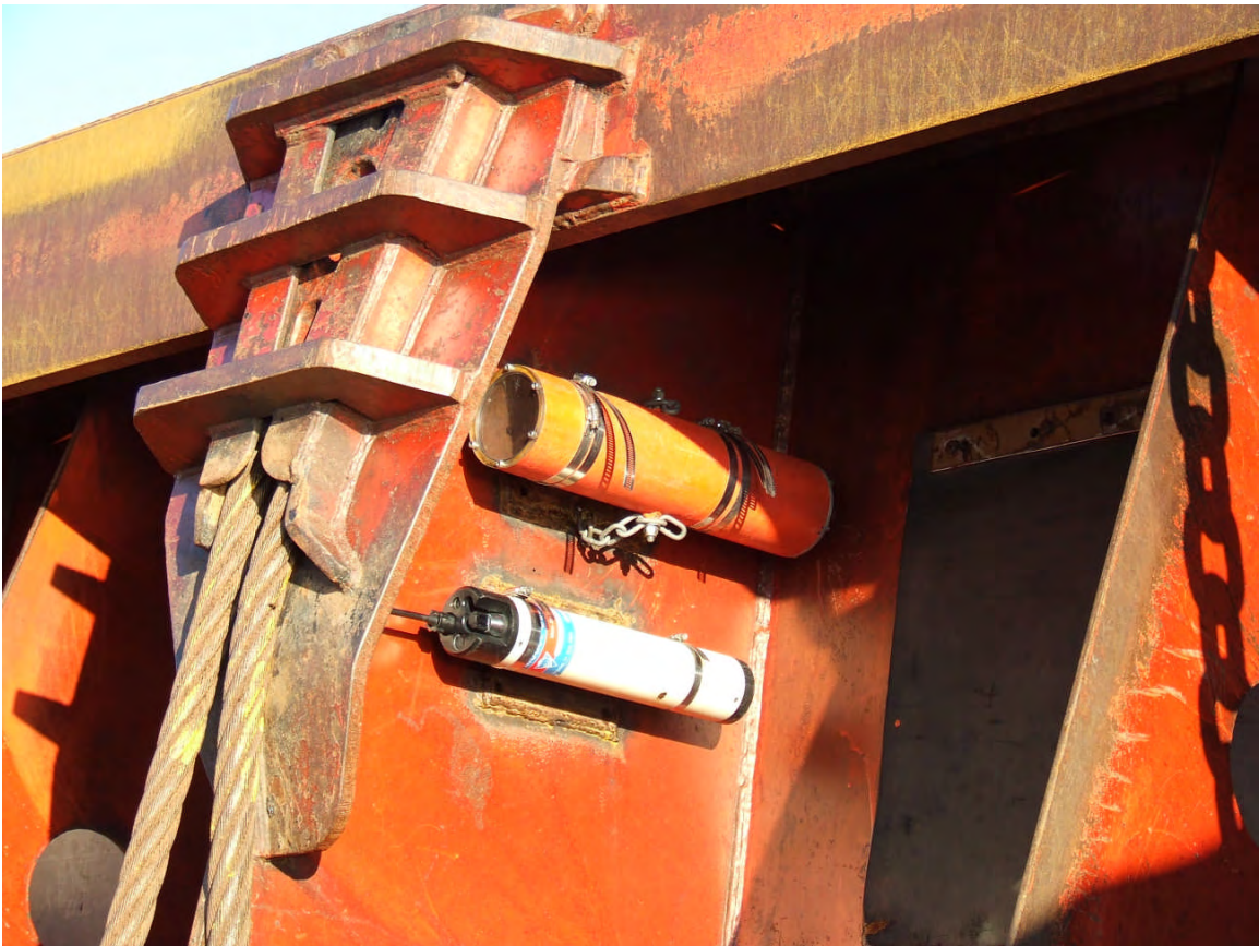
Figure 6. Instrumentation as mounted on the bucket. Upper orange canister contains an accelerometer array. Lower white and black unit is a battery-powered optical backscatter sensor (OBS-3A) with the sensor facing laterally outward from the central bucket support rib and outboard in relation to the bucket's internal axis. When the bucket was closed the instruments were oriented horizontally. When the bucket was open the instruments were oriented at an approximately 45 degree angle from the vertical.
