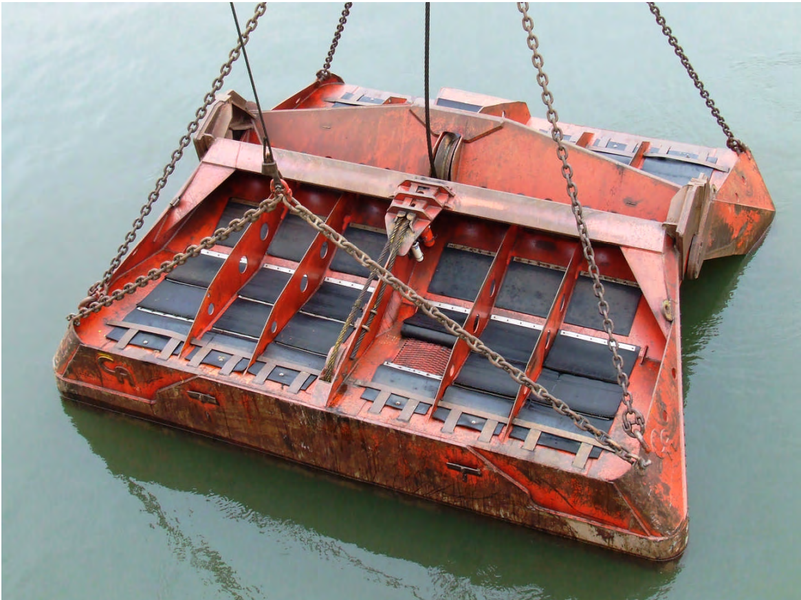
Figure 2. Cable Arm bucket in the open position. Note that the lowest row of vents has been closed by welding metal strips across the flaps.
