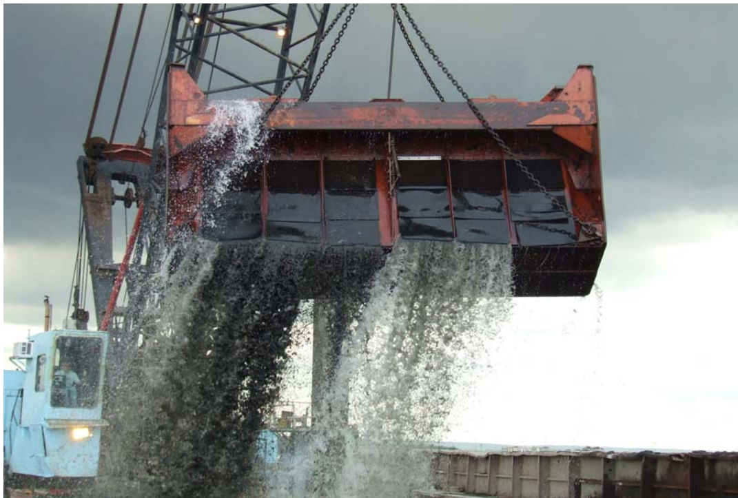
Figure 3. View of the cable arm environmental bucket showing the array of lateral flaps.
