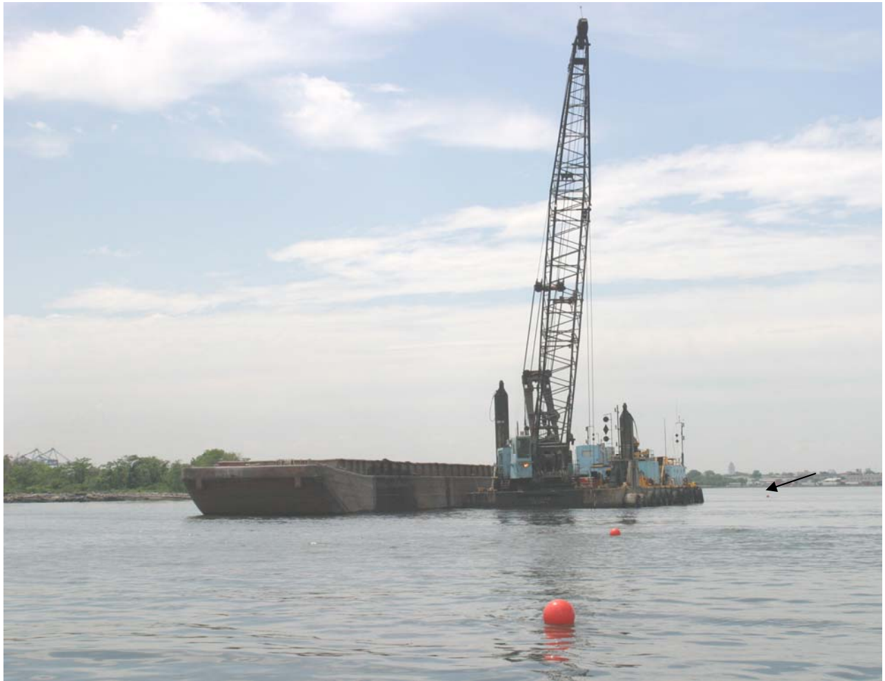
Figure 6. Deployment of fixed buoys with turbidity sensors. In this deployment the tide was carrying the plume toward to foreground. A third buoy with turbidity sensors deployed on the up-current side of the dredge is visible in the background.
