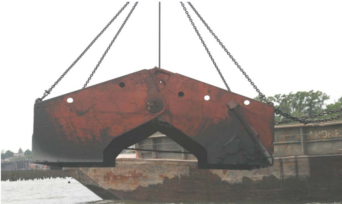
Figure 2. Side view of cable arm environmental bucket in open position.
