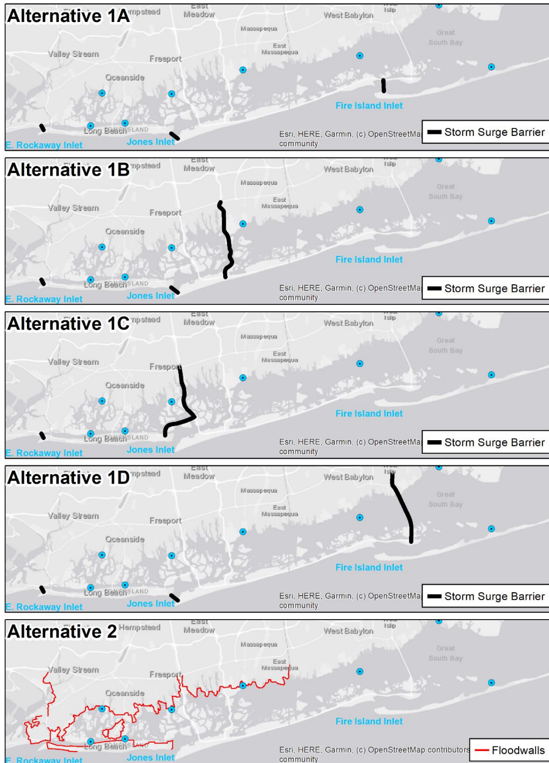
Figure 6-13: Storm Surge Barrier Alternatives
